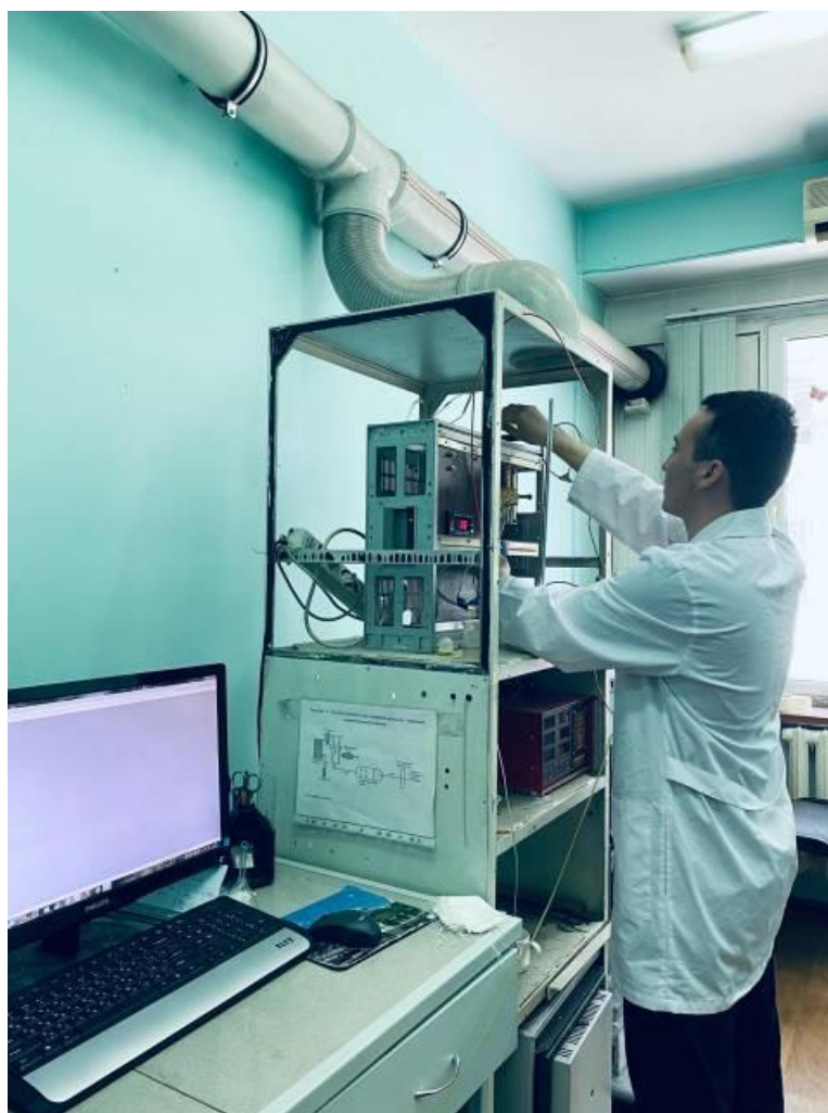
Serkebaev B.S. 1st year Master of Al-Farabi Kazakh National University Conducts testing of synthesized samples in the process of CO 2 adsorption/desorption
